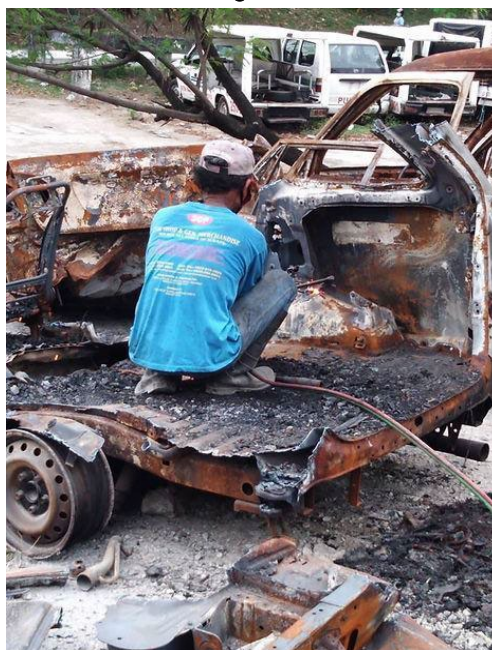
Figure 2.20. Dismantling of Junk Cars, Philippines
